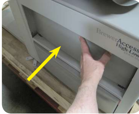
Push top rear pass-through drawer to the right (from a seated patient's perspective).
