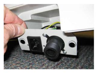
3.Remove three wires connected to the power inlet.
