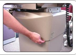
2. The decorative side shroud comes from the factory preadjusted and should fit, or be very close. If fit is too tight loosen the allen screw on the corner that is tight by 1/8 turn. Try fit again. Continue this procedure until it fits correctly.
