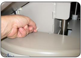
5. Grasp decorative side shroud with both hands and lift straight up. Pull decorative side shroud toward you as you "wiggle" shroud slightly to allow screw heads to pass through the (4) keyhole slots that secure decorative side shroud in place.
