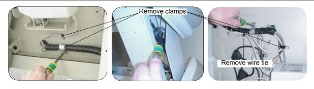
4. Remove the cable clamps and wire tie that secure the actuator cord and the wire conduit to the table's frame.
