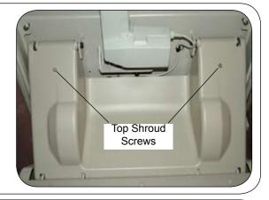
3. Remove two screws and pull the box shroud from table. Set aside screws for re-attachment later.
