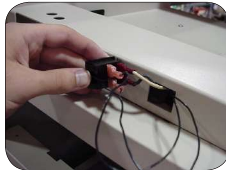
Remove wires from switch
